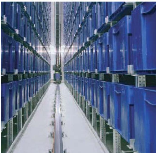
**The mini-loader moves between racking units on both sides of it.**
