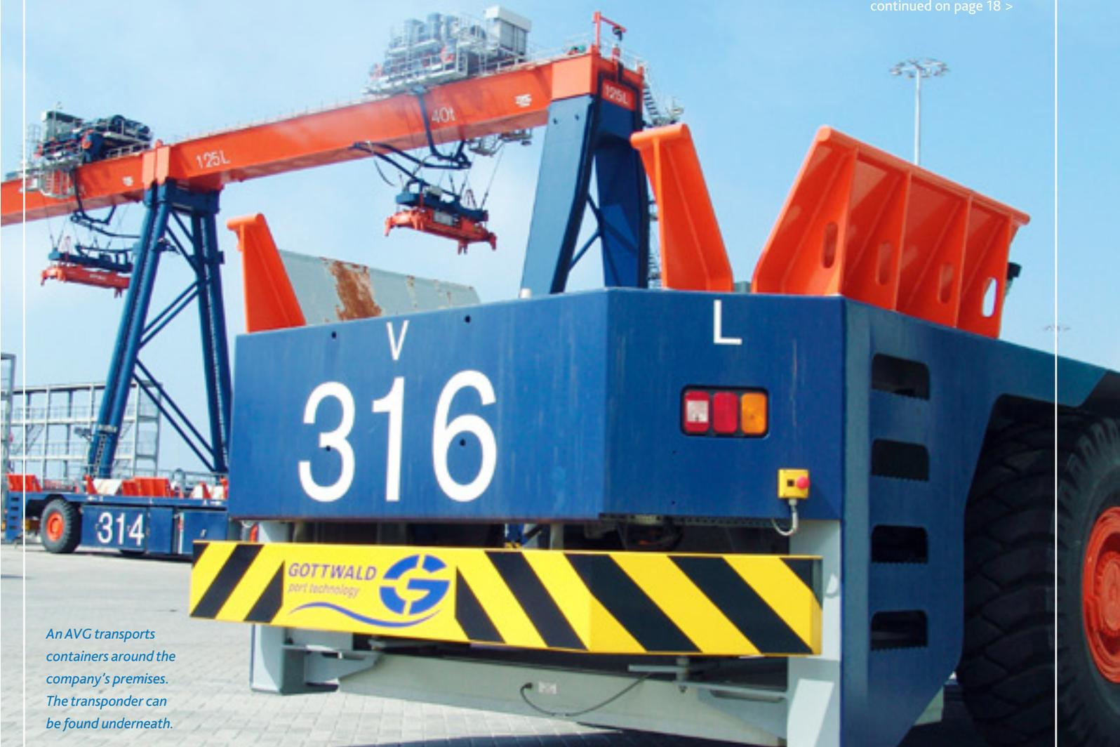
An AVG transports containers around the company's premises. The transponder can be found underneath.
