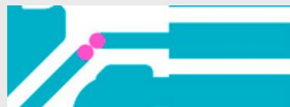
figure 7a - example of missing SM-dam
