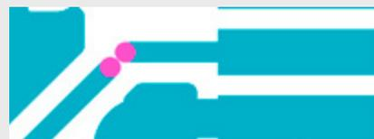
figure 7a - example of missing SM-dam
