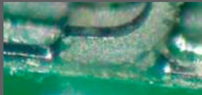
2. the area reserved on the printed circuit board does not match the selected component
