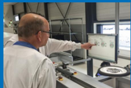
smt-operators (surface mount technology) view line balancing using the Aegis MES-dashboard
