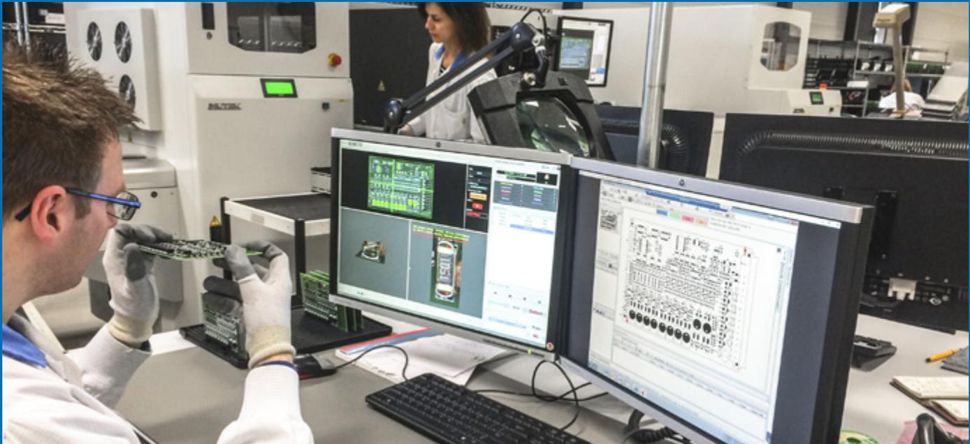
Errors discovered on the inline 3D AOI (Automatic Optical Inspection) were sent by the AOI review station to the Manufacturing Execution System
