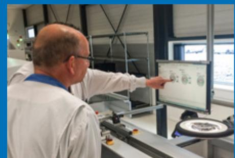
SMT-Operators (Surface Mount Technology) beobachten das Line Balancing mittels des Aegis MES-Dashboards.
